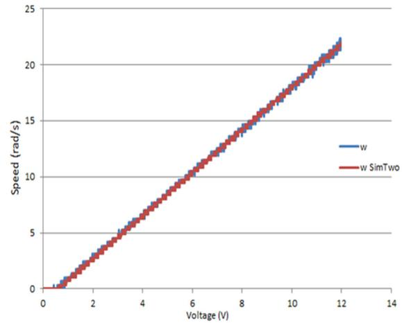
Figure 7 b). Actuator steady state response
